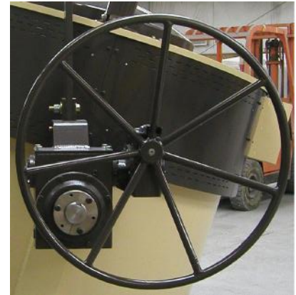
DOUBLE REDUCTION MECHANICAL GEAR BOX FOR PRECISE POURING CONTROL
